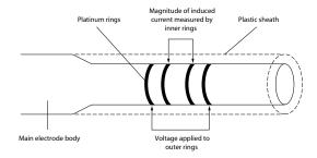
The STCON3 utilizes the 4-ring potentiometric method for measuring conductivity, which incorporates a series of four stainless steel rings formed into the probe shaft. This design completely eliminates polarization, which occurs with the 2-plates amperometric method. Furthermore, without polarization the probe can measure a wider range of conductivity values because it does not suffer from electrolysis.
